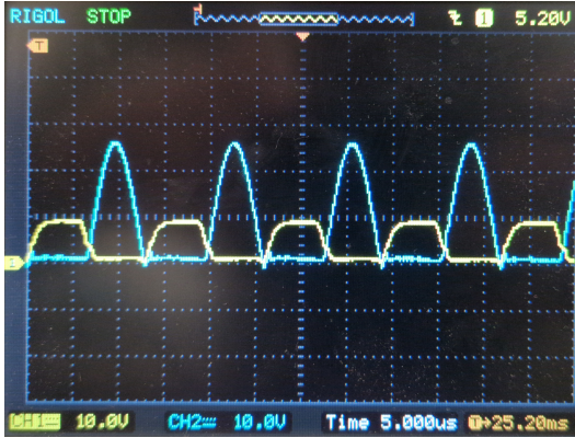
Fig. 4. Self-oscillating inverter waveforms obtained for a main supply voltage of V_{dd} = 10 V. Both the gate (yellow) and drain (cyan) voltages of MOSFET M1 are measured. The peak drain voltage is 27 V, while the gate voltage is limited to 10 V by the Zener diodes. The measurements are made with the rectifier and the incandescent lamp connected to the secondary of the WPT transformer. Under these conditions, the oscillation frequency f_0 is 80 kHz.
